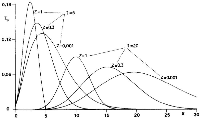
FIG. 2. Solid temperature distribution for different values of  $t$  and  $z$ , due to an impulse inlet fluid temperature.
