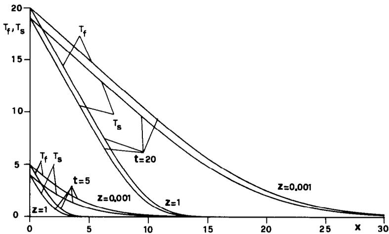
FIG. 6. Fluid and solid temperature distributions for different values of  $t$  and  $z$ , due to a ramp inlet fluid temperature.
