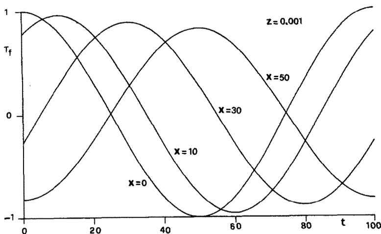
FIG. 7. Fluid response to a cosinusoidal inlet temperature for different values of  $x$ .
