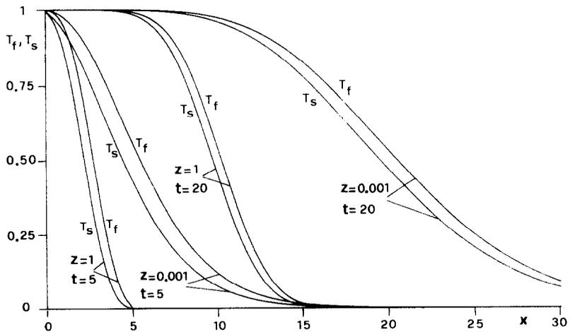
FIG. 4. Fluid and solid temperature distributions for different values of  $t$  and  $z$ , due to a step inlet fluid temperature.
